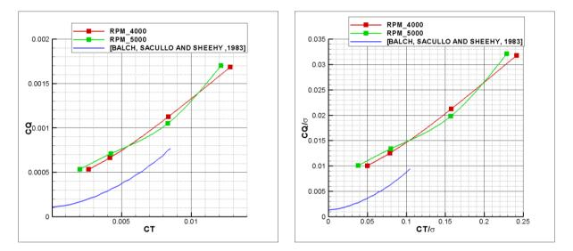
Figure 7:  $C_Q$  versus  $C_T$  curves and  $C_q/\sigma$  versus  $C_t/\sigma$  curves
