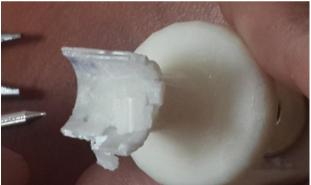
a) Cracks before the damage b) Cracks after the damage Figure 5: Cracks on the Hub for Baseline I
