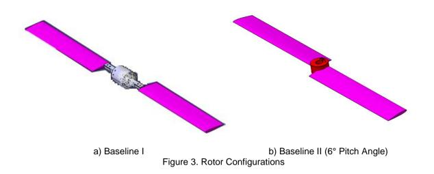
The radius, area and solidity values of the rotor of Baseline II configuration are given in Table 2. Solidity is basically the ratio of the total blade area to rotor disk area.
